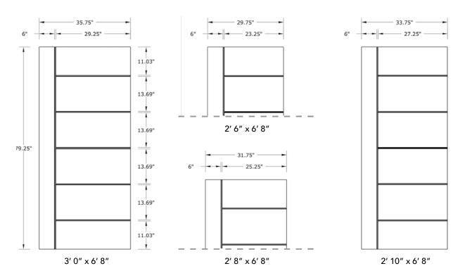
NOTE: BY REQUEST, DOOR HEIGHT COMES IN VARYING DIMENSIONS TO A MINIMUM OF  $79^{\circ\circ}$ . EXCESS WILL BE TAKEN FROM BOTTOM RAIL. ALL OTHER DIMENSIONS WILL REMAIN THE SAME.
